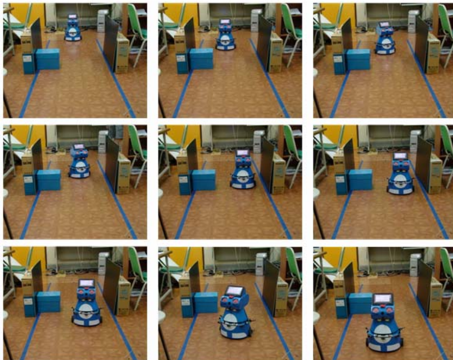
Fig. 10 The successive images when the robot navigates collision-free in the passage.
