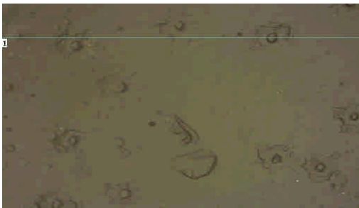
Fig. 2. One of the images of the top surface of the 14-inch wedged LGP measured by the 3D laser microscope VK-8700.
