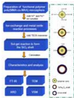
Fig. 1. Flow chart of synthesis and experiments for NiFe 2 O 4 /SiO 2 hollow spheres.
