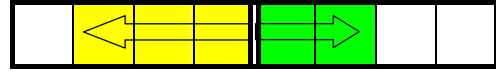
Figure 4: n=8 . The query \text{Sum}(A[1] : A[5]) can be divided into two sub-queries \text{Sum}(A[3] : A[1]) and \text{Sum}(A[4] : A[5])
